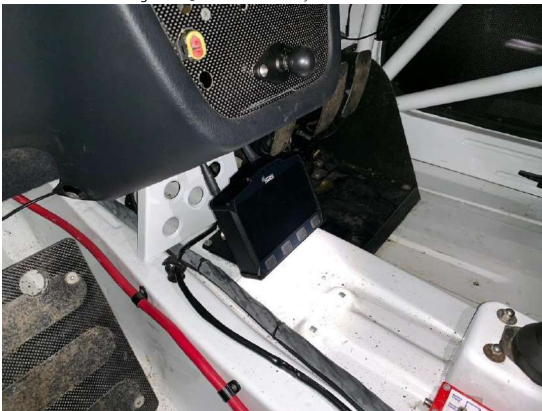
Figure 2. The WRC tracking unit mounted onto the 25mm rubber ball mount and connected through the RallySafe connector
