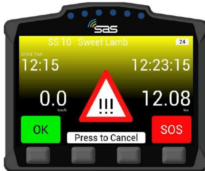
SCREEN 15. Manual Hazard in Transport Mode
